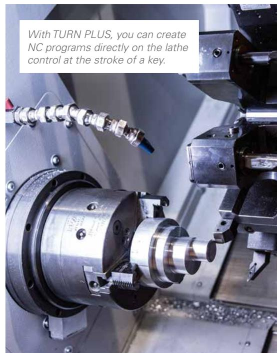
*With TURN PLUS, you can create NC programs directly on the lathe control at the stroke of a key.*
