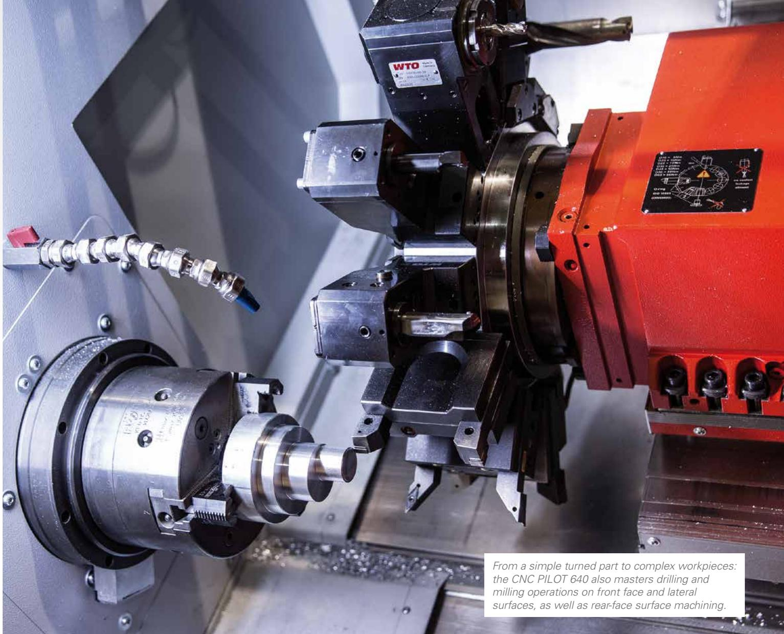
*From a simple turned part to complex workpieces: the CNC PILOT 640 also masters drilling and milling operations on front face and lateral surfaces, as well as rear-face surface machining.*
